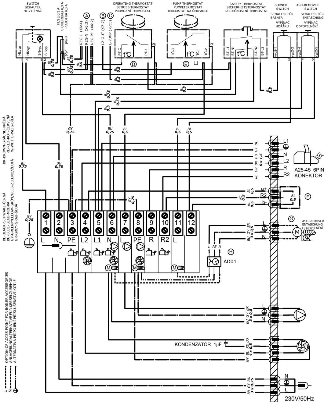
**WHEN USE ELECTRONIC REGULATION ACD01 AND PELLETBURNER A25-45 MUST BE THESE CHANGES OF WIRING:
